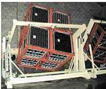
These "portable" gyropalettes may hold over 3,000 bottles. Note the palette on the right is more upright, indicating it is farther along in the riddling process.
